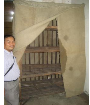
Box-type EC 1.3x0.9x2.0 m in L, W, H, with moist jute sack
