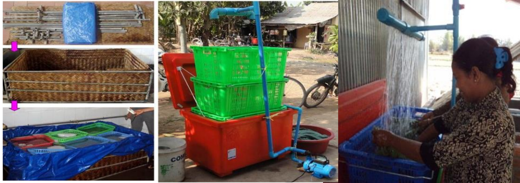
រូបភាពទី២១ Simple knockdown hydrocooler (leftmost) and overhead hydrocooler applying cold water with water pump on the produce (middle and rightmost).
