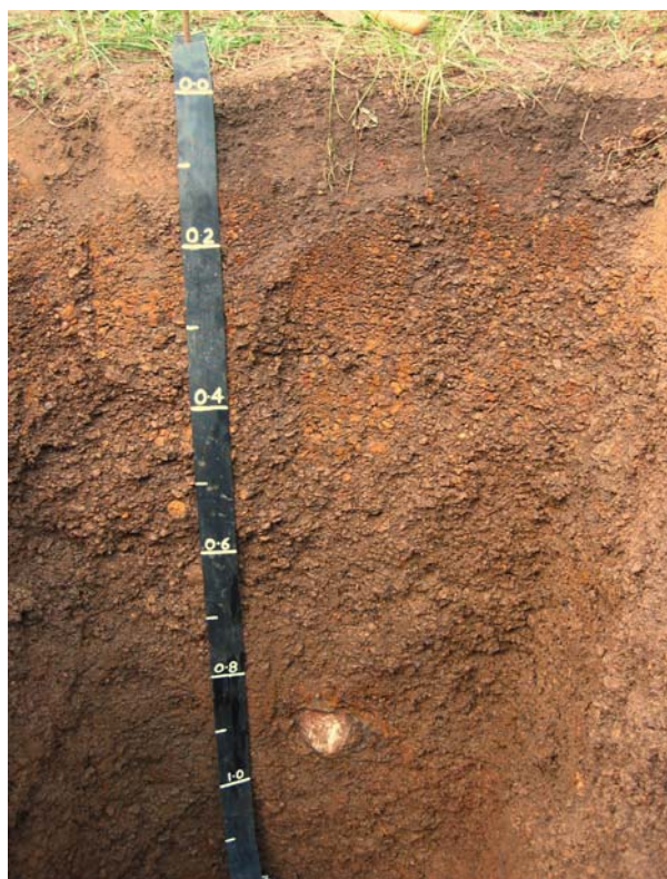
Figure 3. Typical profile for Ou Reang Ov Soil group in Ou Reang Ov district, Kampong Cham province. Note the abundance of ferruginous gravel from about 15 cm depth and below, and the basalt rock at 90 cm depth.
